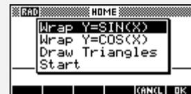
**Wrap Y=SIN(X)** graphs the unit circle and one period of the sine curve. The calculator is automatically in TRACE mode. Using the left and right arrows, the student can trace around the unit circle. The up and down arrows will move the cursor to the other curve.
